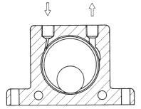
Housing made from extruded aluminium alloy Hardened guides made of steel Nylon end plates Hardened ball
