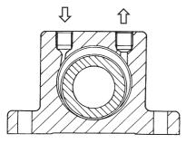
Housing made from extruded aluminium alloy Highly flexible steel guides Cast precision steel roller Special bronze end plates
