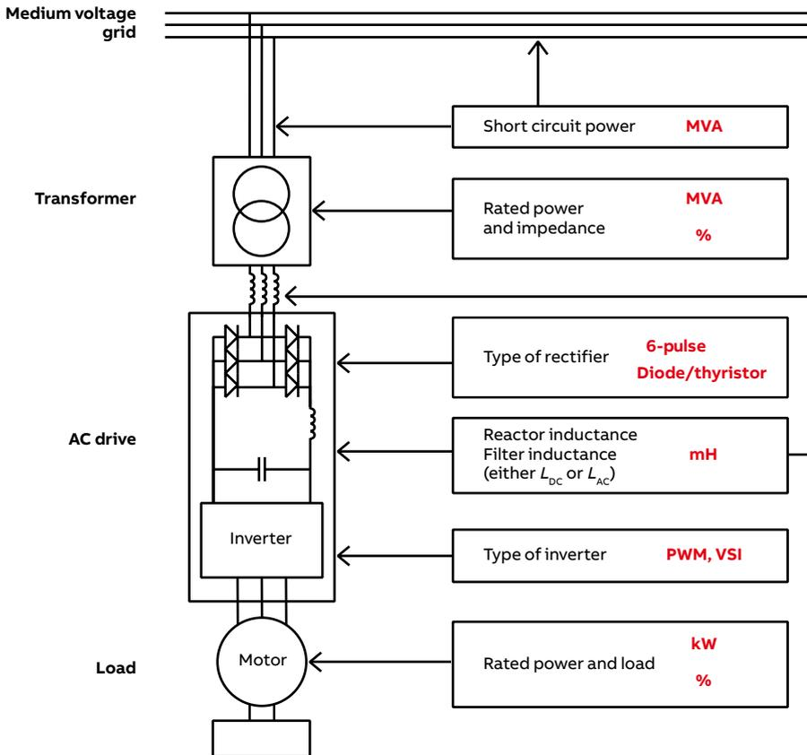
Harmonics reduction can be achieved either by structural modifications in the drive system or by using external filtering. The structural modifications may be to strengthen the supply, or to use 12 or more pulse drives, to use a controlled rectifier, or to improve the internal filtering in the drive.
