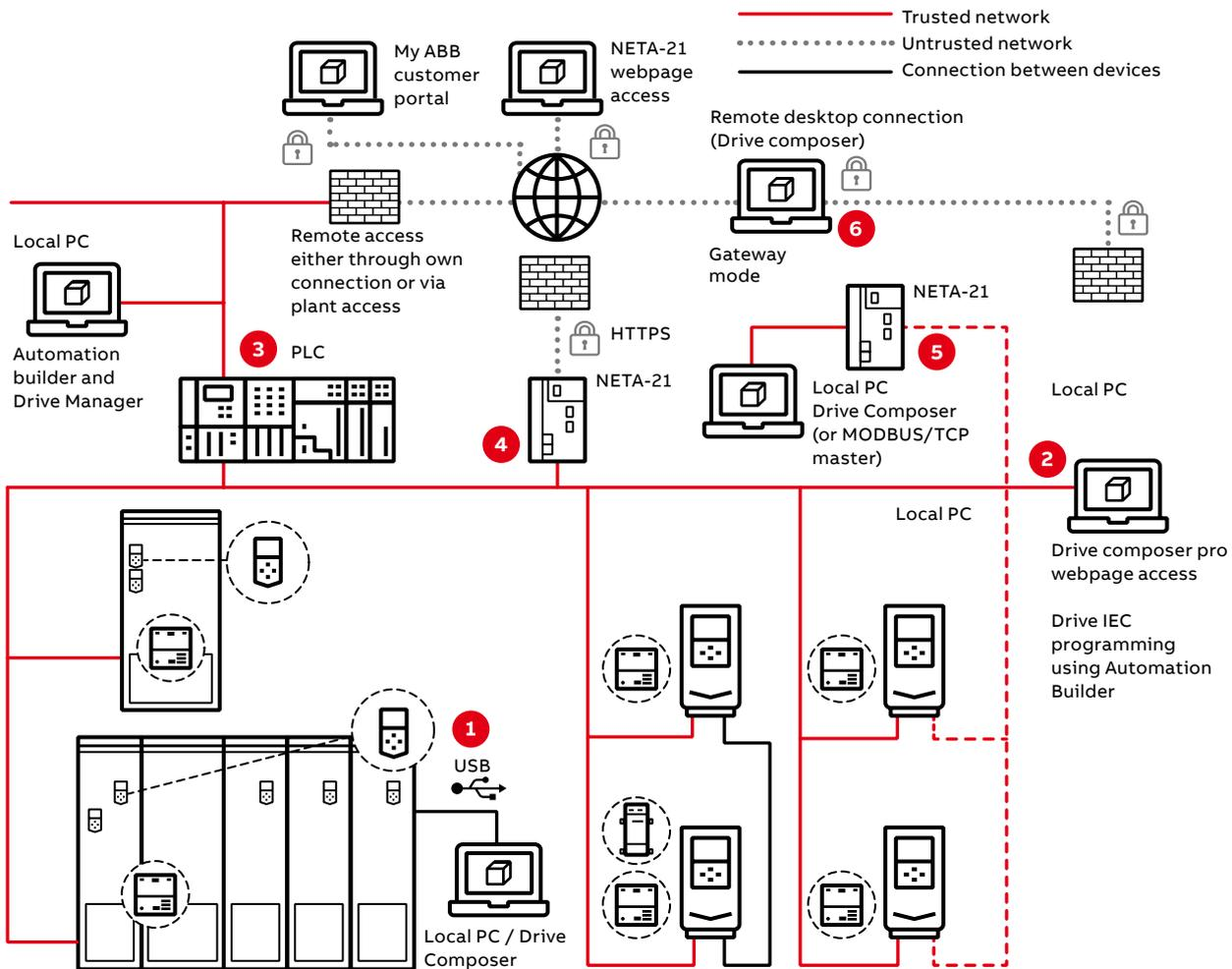
1. Local connections (point-to-point serial communication, e.g. USB) or
