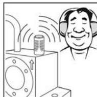
6. The ball bearings are lubricated for life. Oiled air however will not harm the operation of the GT-vibrator.
