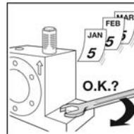
5. If you notice a loss of power of the vibrator or if it even stops, then remove the silencer. If the vibrator operates now, wash out the silencer or replace it.
