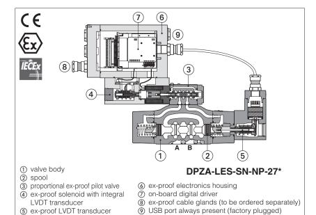
Ex-proof digital servoproportional directional valves, piloted with two LVDT position transducers (pilot valve and main stage) and zero spool overlap for position closed loop controls.
