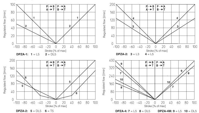
Note: Hydraulic configuration vs. reference signal for configurations 60 and 70 (standard and option /B)
