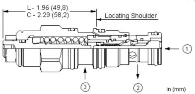
Counterbalance valves with pilot assist are meant to control an overrunning load. The check valve allows free flow from the directional valve (port 2) to the load (port 1) while a direct-acting, pilot-assisted relief valve controls flow from port 1 to port 2. Pilot assist at port 3 lowers the effective setting of the relief valve at a rate determined by the pilot ratio.
