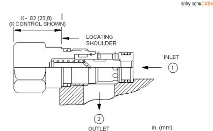
Free-flow, nose-to-side check valves are on/off circuit components that allow free flow from the inlet (port 1) to the outlet (port 2) and block flow in the opposite direction.
