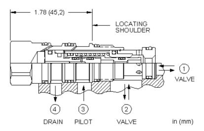
This is a normally open, balanced poppet, switching element. Pilot pressure at port 3 shifts the valve to the closed position.
