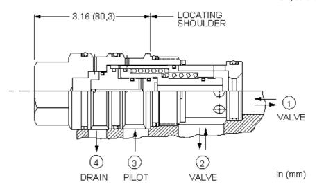
This is a normally open, balanced poppet, switching element. Pilot pressure at port 3 shifts the valve to the closed position.
