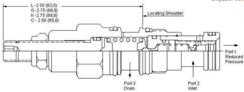
Pilot-operated, pressure reducing valves reduce a high primary pressure at the inlet (port 2) to a constant reduced pressure at port 1, allowing circuits with multiple pressure requirements to be operated using a single pump.
