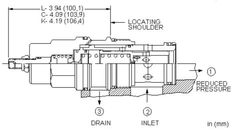
Pilot-operated, pressure reducing valves reduce a high primary pressure at the inlet (port 2) to a constant reduced pressure at port 1, allowing circuits with multiple pressure requirements to be operated using a single pump.
