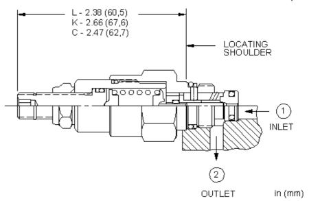
Two-port, pilot-stage, direct-acting relief cartridges are fully adjustable, normally closed pressure regulating valves. When the pressure at port 1 (inlet) is sufficient to overcome the spring force (valve setting), a flow path is opened from port 1 to port 2 (tank).
