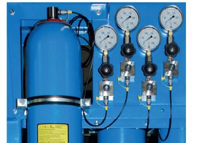
Diaphragm accumulator with mini-measuring connection
